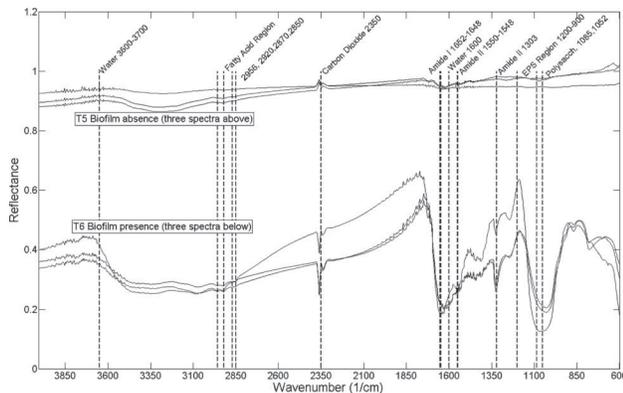
Figure 5. T5, T6 representative FTIR spectra with biofilm peaks.
