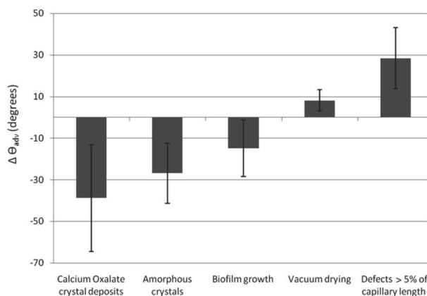
Figure 4. Impact of surface fouling conditions on  $\Delta \theta_{adv}$  with 95% confidence intervals.
