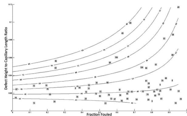
Figure 7. Comparison of  $\theta_{adv}$  from Equation (1) (contour lines) with experimental data (shaded boxes) for give ranges ( $0.001 \leq f_{fouled} \leq 0.961$ ,  $0.009 \leq d/l_{cap} \leq 0.117$ ).
