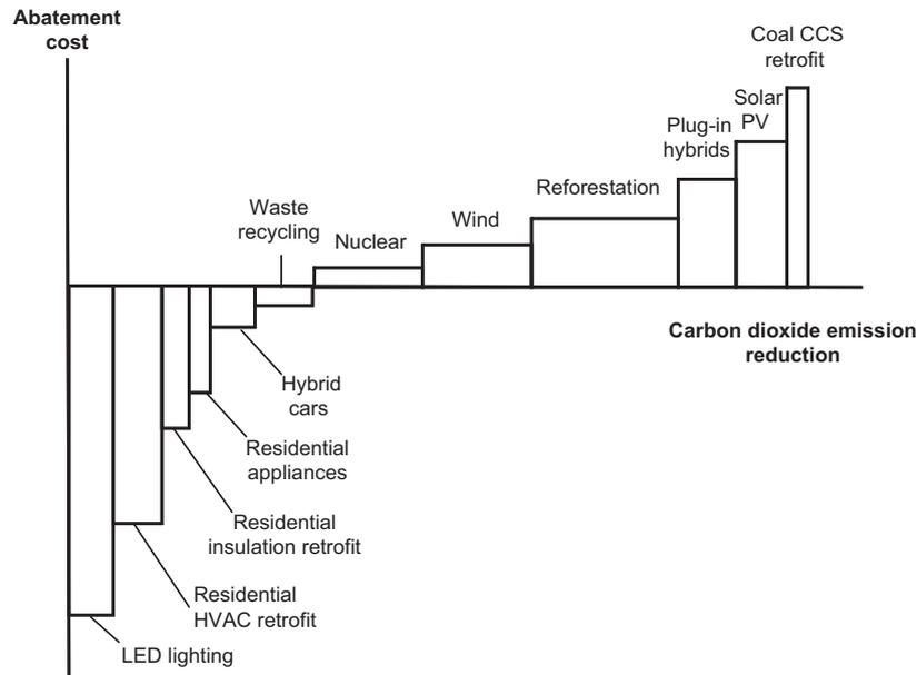
**Figure 2.** Simplified, schematic McKinsey diagram showing carbon dioxide abatement costs and benefits (after Enqvist *et al.*, 2007); CCS, carbon dioxide capture and geological storage; HVAC, heating, ventilation and air conditioning; LED, light-emitting diode; PV, photovoltaic
