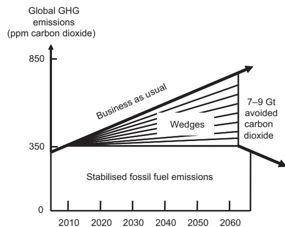
Figure 1. Schematic diagram, after Pacala and Socolow (2004), illustrating how 'wedges' of avoided carbon dioxide emissions can help keep down atmospheric carbon dioxide
