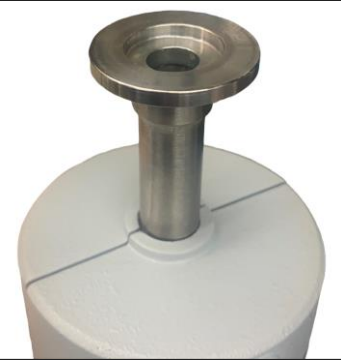
Opening of Baratron incompatible with tube connections
