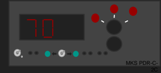
MKS PDR-C-2C Power Supply Readout: Displays pressure coming from Baratron
