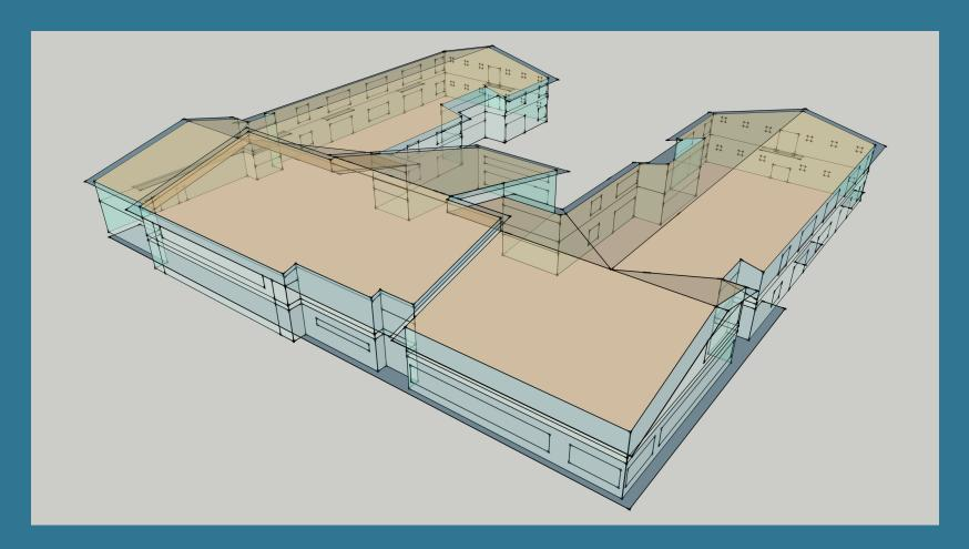
Assign entity types to appropriate SketchUp model parts (Sefaira recognizes 7 entity types: floor, wall, internal wall, party wall, roof, glazing and shading).
