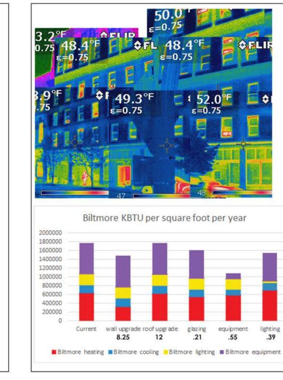
The majority of the heat loss is through the storefront windows on the ground floor, and thermal losses also occur at the floor plate.
