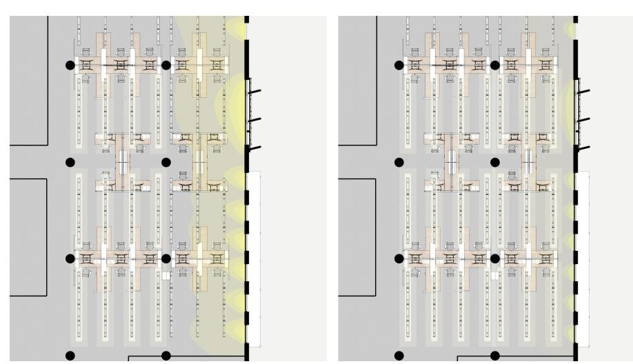
A smarter lighting design will help to provide even adequate lighting throughout the day, without over exposing those by the window or leaving others in the dark. Having lights running parallel to the exterior wall and set to different controls will allow for artificial lighting to be used by the window only when the sunlight in not sufficient.
