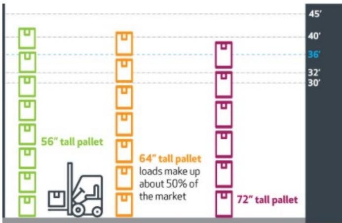
*In a building with a 36-foot clear height, a user will be able to rack one pallet position higher. Fifty-six inch pallets require 37 feet clear before they can gain another pallet position.*
