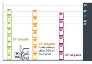
In a building with a 36-foot clear height, a user will be able to rack one pallet position higher. Fifty-six inch pallets require 37 feet clear before they can gain another pallet position.
