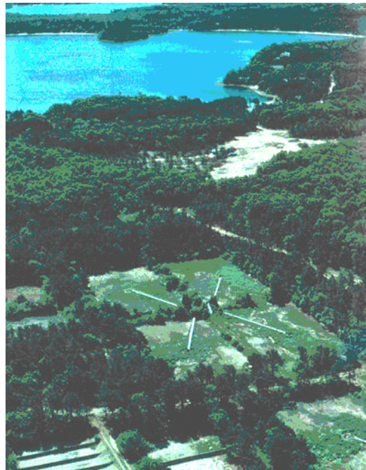
Treated wastewater disposal beds, which created a large subsurface plume of contaminated ground water ( toxics.usgs.gov/photo_gallery/capecod.html )
