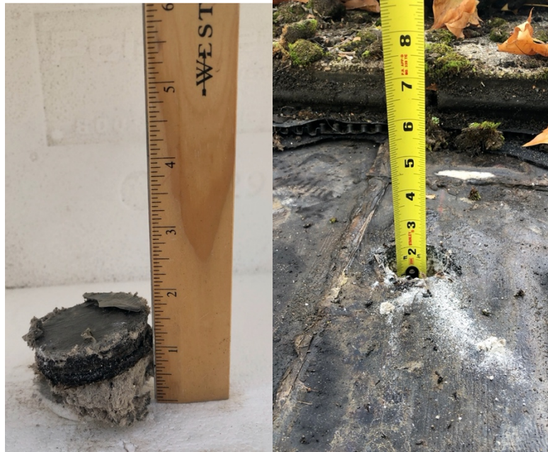
Roof core on the north end of roof J tested negative for asbestos
