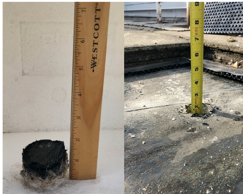
Roof core on the north end of roof J tested negative for asbestos
