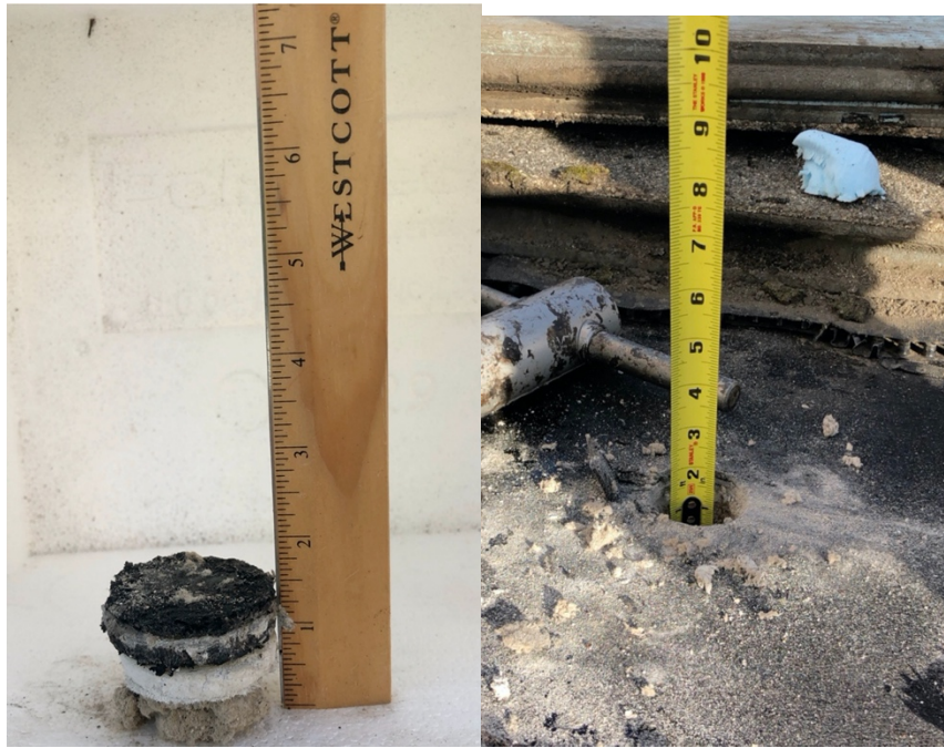
Roof core on the north end of the north portion of roof N tested negative for asbestos
