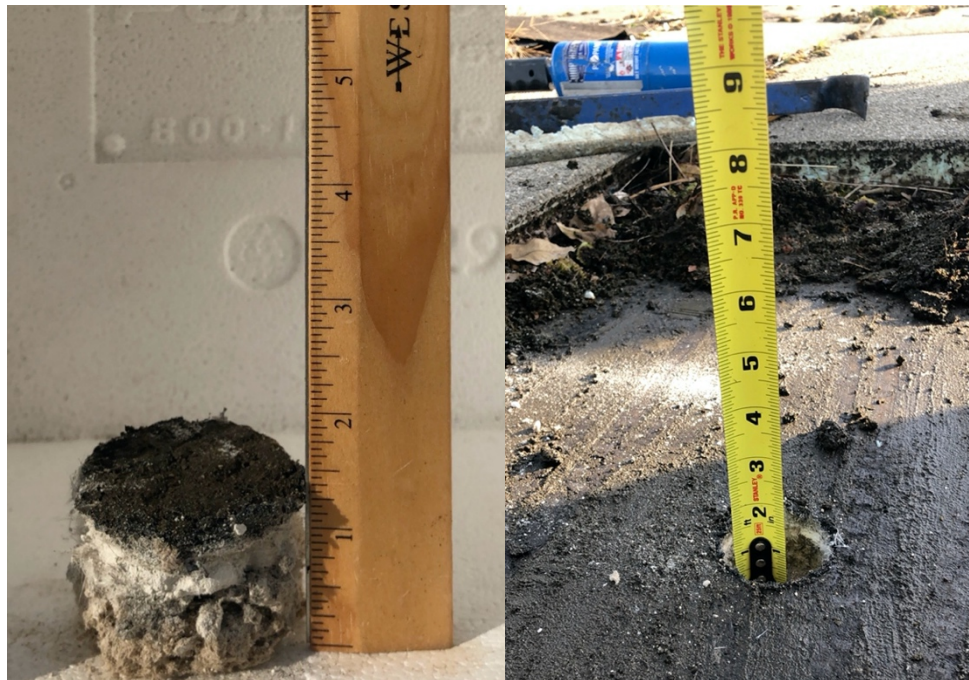
Roof core on the south end of roof J tested negative for asbestos
