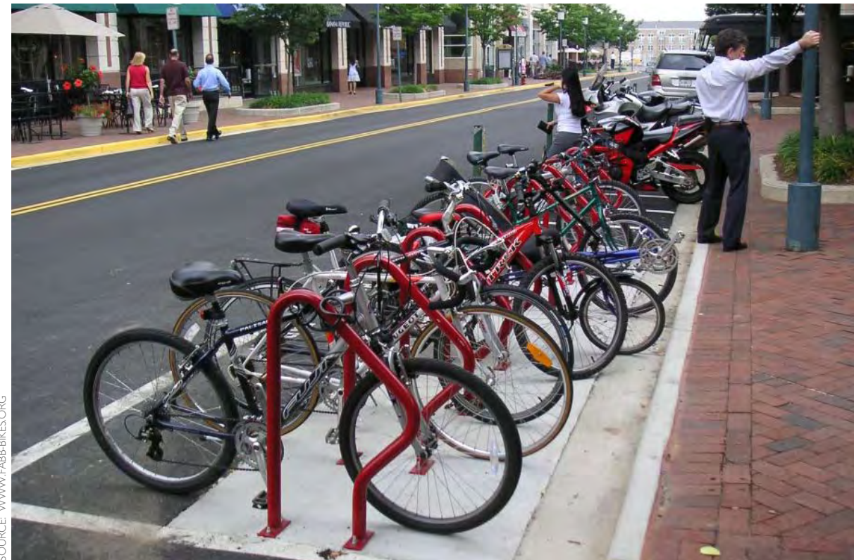
Bike racks replace on-street car parking.
