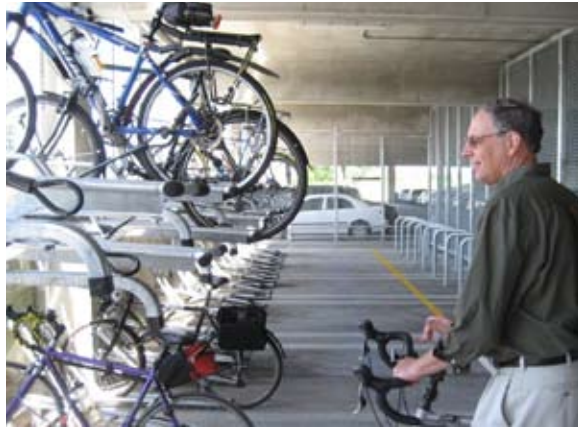
In late summer 2010 TriMet opened the Bike & Ride facility at the Sunset Transit center, removing 8 car parking spots to provide 74 bike spaces available to registered users for a small fee. Image source: Oregonlive.com.
