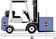
A forklift's front axle serves as a fulcrum, balancing the forklift and the load.
